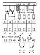
The data terminals are used for connection of e.g. a PC. The signal is passive and galvanically separated by means of optocouplers. Conversion into RS232 level requires connection of data cable 66-99-106 (D-Sub 9F) or 66-99-098 (USB) using the following connections:
